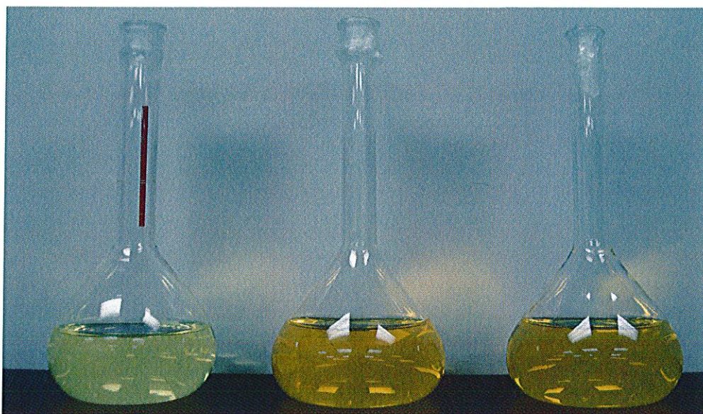
Figure 14. The three phosphorus-containing solutions, K_4[\alpha\text{-PV}^V\text{W}_{11}\text{O}_{40}] , \text{Cs}_6[\alpha\text{-1,2,3-PV}_3\text{W}_9\text{O}_{40}] , and \text{Cs}_5[\gamma\text{-PV}_2\text{W}_{10}\text{O}_{40}] , made for IC and ^{13}\text{P} NMR analysis.
