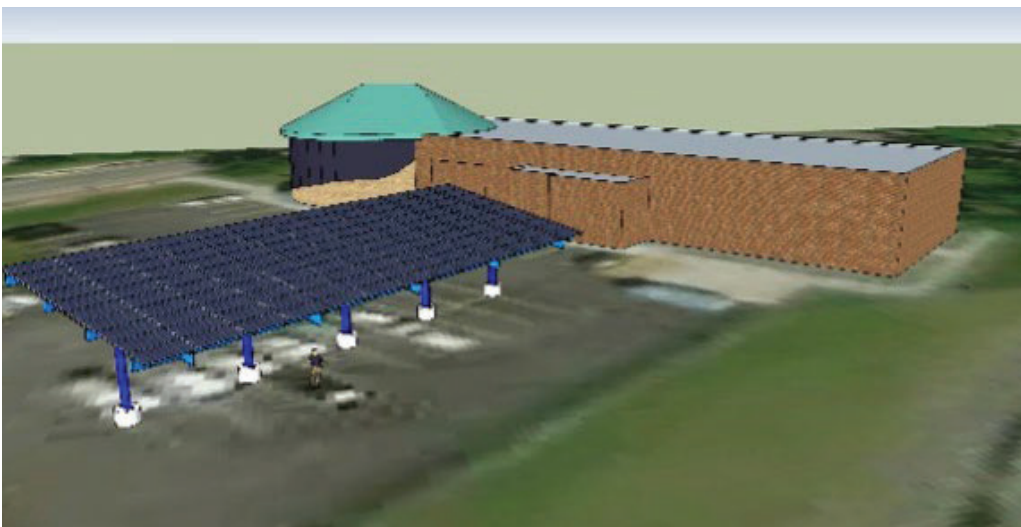
Rendering of possible carport solar Photo Voltaic array in American Indian Resource Center Parking Lot
